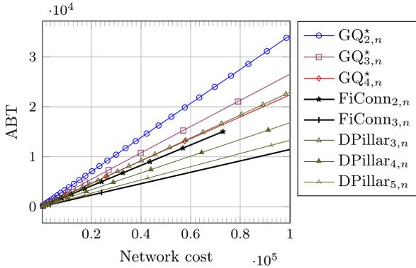
Fig. 7. ABT in terms of network cost for  $GQ^*$ -routing, TOR, and DPillarSP, where a DCN DPillar is 110% the cost of a DCN  $GQ^*$  with the same number of server nodes, whilst a DCN FiConn is 98% of the cost of a DCN  $GQ^*$ . Network cost is normalised by the aggregated component cost per server in  $GQ^*$ .
