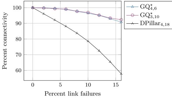
Fig. 9. Routed connectivity of  $GQ^*$ -routing and  $DPillarMP$ .
