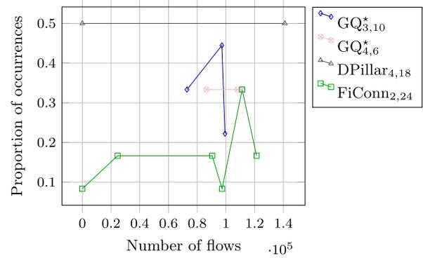
**Fig. 15.** Histogram of proportion of flows per link under the all-to-all traffic pattern. The mean number of flows per link are 89,567, 101,953, 84,615, and 141,187, for GQ\*<sub>3,10</sub>, GQ\*<sub>4,6</sub>, FiConn<sub>2,24</sub> and DPillar<sub>4,18</sub>, respectively. Connecting lines are drawn for clarity.
