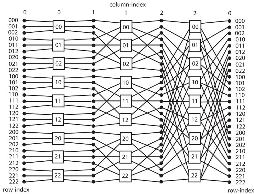
**Fig. 2.** A visualization of DPillar<sub>3,6</sub>. Squares represent switch-nodes, whereas dots represent server-nodes. For the sake of simplicity, the left-most and the right-most server-columns are the same (server-column 0).
