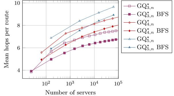
Fig. 11. Routed ( $GQ^*$ -routing) and unrouted mean-distance in  $GQ^*$  with 10% link failures.
