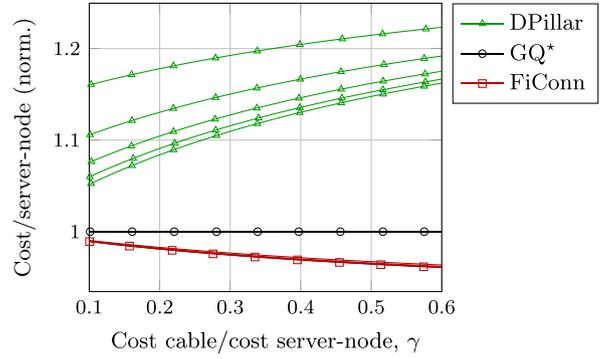
**Fig. 4.** The component costs per server-node of FiConn and DPillar, relative to that of GQ\*, for  $\rho \in \{0.01, 0.02, 0.4, 0.8, 1.6\}$ .
