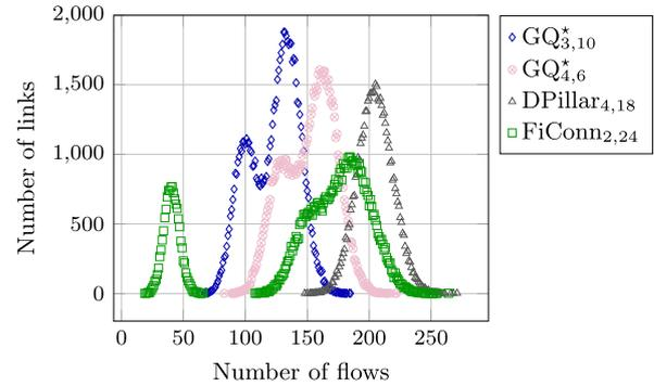
**Fig. 16.** Distribution of number of flows per link for the random traffic pattern. Not plotted are 52,488 unused links in DPillar and 6,162 unused links in FiConn.
