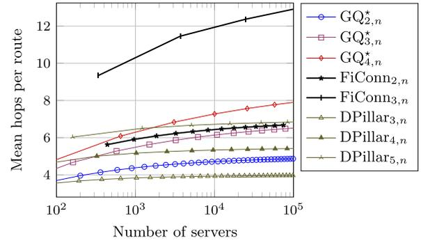
Fig. 8. Routed mean hop-distances for  $GQ^*$ -routing, TOR, and DPillarSP.
