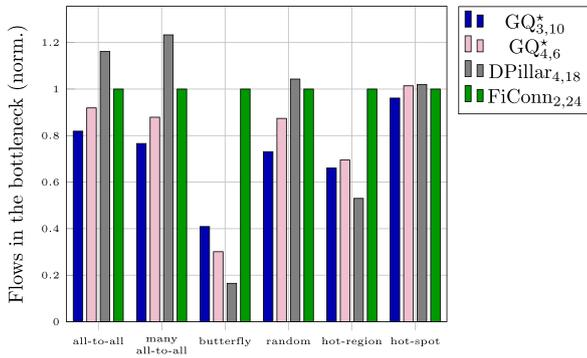
**Fig. 13.** Relative number of flows in the bottleneck for the different traffic patterns, normalised to FiConn and TOR.
