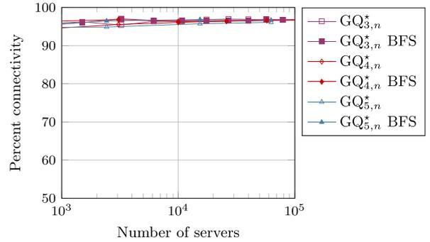
Fig. 12. Routed ( $GQ^*$ -routing) and unrouted connectivity of  $GQ^*$  with 10% link failures.
