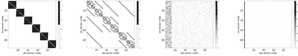
**Fig. 5.** Representative trace matrices for a 96-server-node DCN. From left to right: many all-to-all, butterfly, hot-region, and hot-spot. The many all-to-all traffic pattern is applied to a random permutation of the server-nodes, and is drawn unshuffled here only for clarity.
