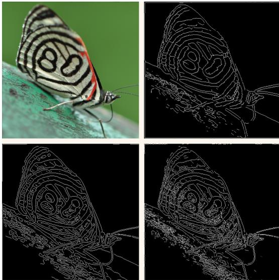
Figure 8. Edge maps for Butterfly.bmp (top-left); ours (top-right), Canny's (bottom-left) and Prewitt's (bottom-right)
